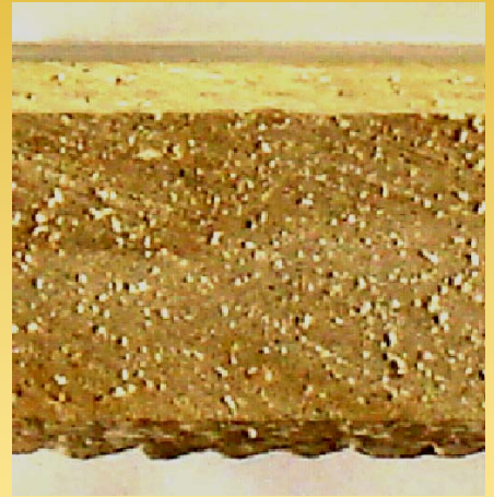
Cross section of sandwich panel construction
